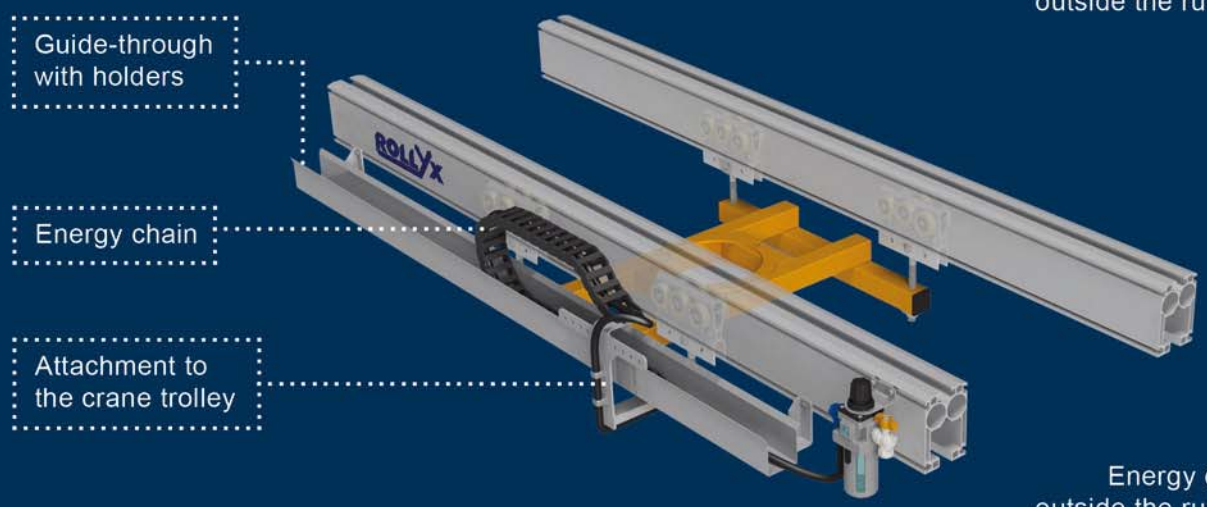
Energy feeding in C-rail outside the runway
